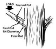
NOTE: For second and final cuts (from top of limb of branch), hold font cutting guide against the limb being cut. This will help steady the limb and make it easier to cut. Allow chain to cut for you. Exert only low downward pressure. If you force the cut, damage to the bar, chain or motor can result.
