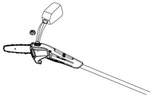
NOTE: Do not use dirty, used or contaminated oil. Damage may occur to the bar or chain.
